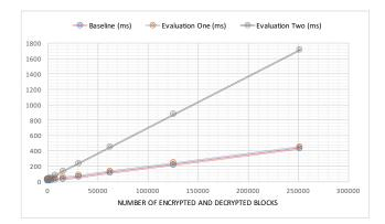
Figure 4: Performance evaluation of AES sample code. For evaluation two, processing of one data block (for encryption and decryption) leads to two SGX ECALLS.
